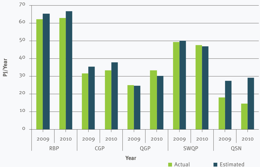
Figure 20 Actual and estimated throughput of major Queensland pipelines, 2009 and 2010 (PJ/year)
